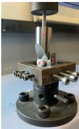
**Figure 2.** Shearing rod (a), The plate of pure iron (b), Titanium disc (c), Zirconia disc (d), Shear bond testing (e)
