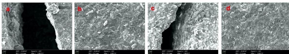
**Figure 4.** Scanning electron microscope (SEM) images of Al<sub>2</sub>O<sub>3</sub> sandblasted roughened titanium surfaces at a magnification of 5000'. (a) GC FujiCEM Evolve; (b) G-CEM LinkForce; (c) GC Fuji I; (d) G-CEM ONE.
