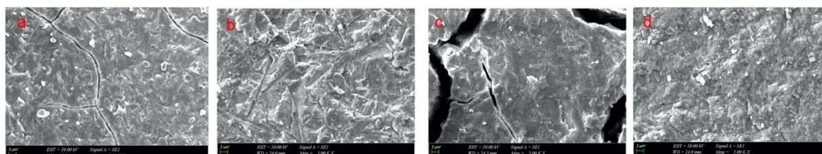
**Figure 5.** Scanning electron microscope (SEM) images of titanium surfaces treated with CoJet at 5000' magnification. (a) GC FujiCEM Evolve; (b) G-CEM LinkForce; (c) GC Fuji I; (d) G-CEM ONE.
