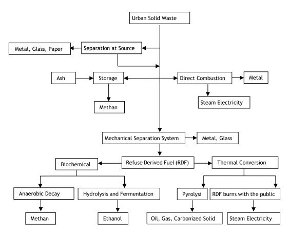
Figure 1. Energy production technologies of urban solid wastes [8].
